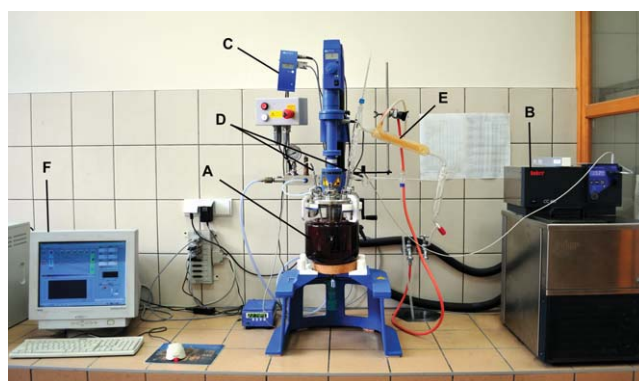
Figure 1 The IKA® LR 2000 system; (A) reactor vessel, (B) heating circulator bath, (C) torque measuring instrument, (D) temperature sensors, (E) Dean-Stark distillation trap, (F) PC with Labworldsoft® software. [Color figure can be viewed in the online issue, which is available at wileyonlinelibrary.com ]
